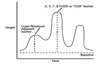
RESPONSE or INSTRUMENTAL RESPONSE - A measurement of the output of the High Resolution Gas Chromatograph/High Resolution Mass Spectrometer (HRGC/HRMS) detector in which the intensity of the signal is proportionate to the amount (or concentration) detected. Measured by peak area or peak height.
