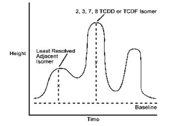
RESPONSE or Instrumental Response - A measurement of the output of the HRGC/HRMS detector in which the intensity of the signal is proportionate to the amount (or concentration) detected. Measured by peak area or peak height.
