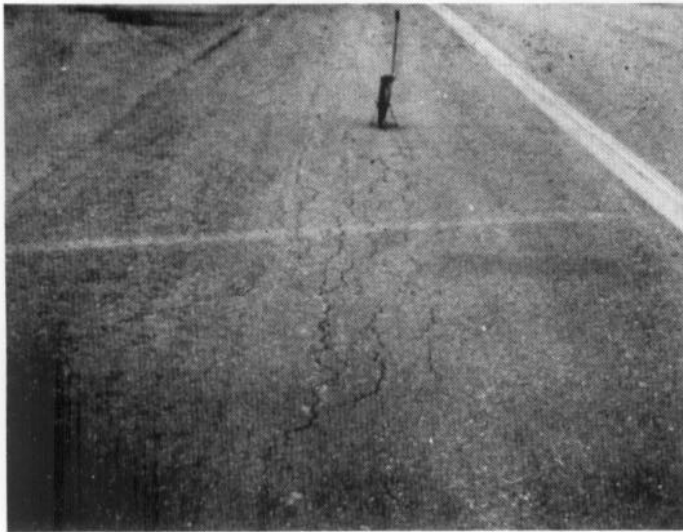
Figure 2. Low severity alligator cracking
